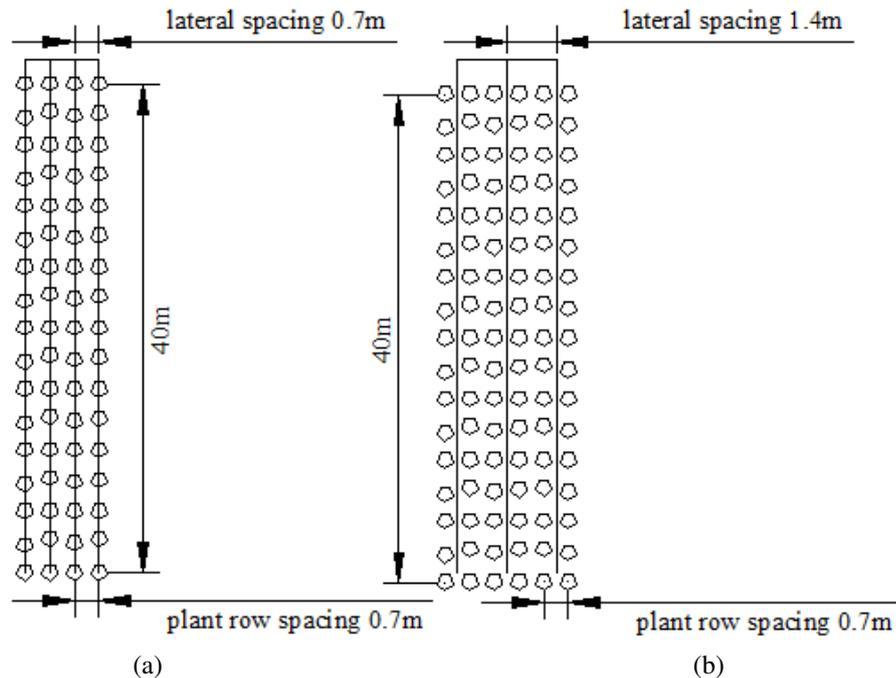
Figure 1. Design of lateral pipe for each crop row (a) and each two crop rows (b).
