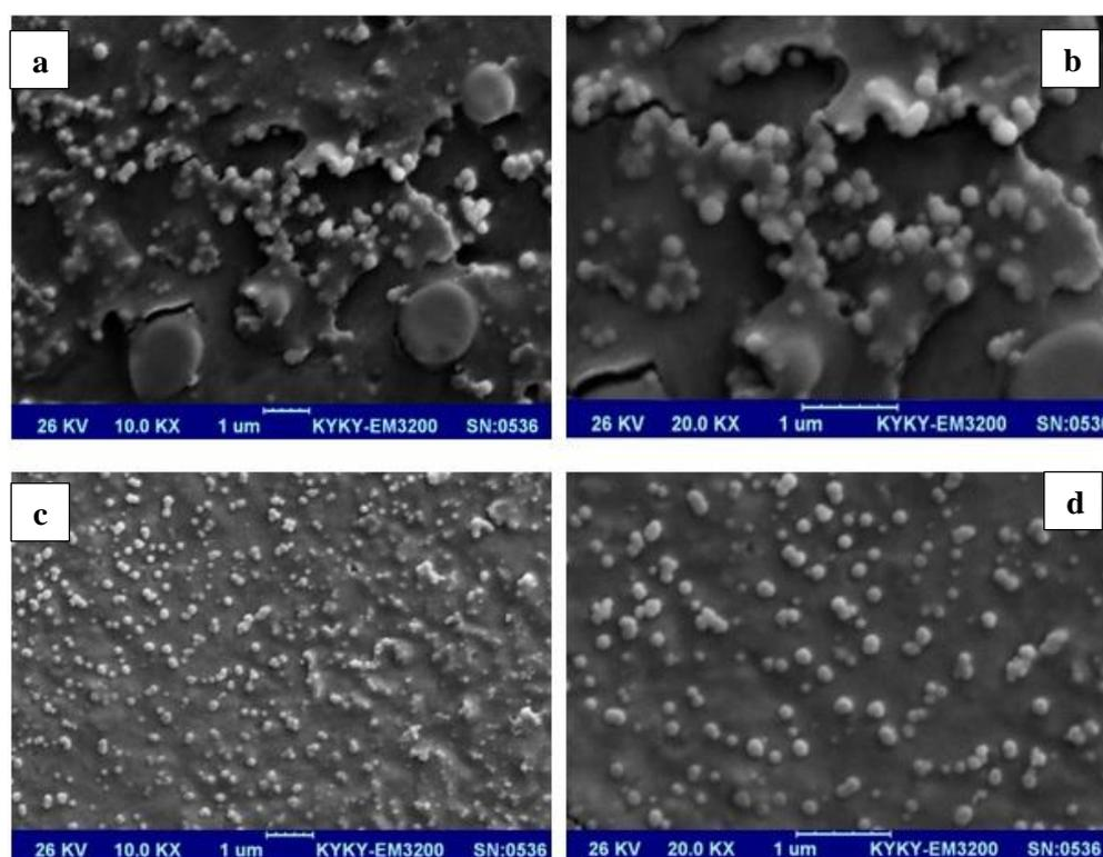
**Figure 3.** SEM image at 26 kV of: (a) Chitosan nanoparticle (10,000X); (b) Chitosan nanoparticle (20,000X); (c) Thyme essential oil loaded chitosan nanoparticle prepared using an initial weight ratio of chitosan: thyme essential oil of 1: 0.4 (10,000X), and (d) 1: 0.4 (20,000X).
