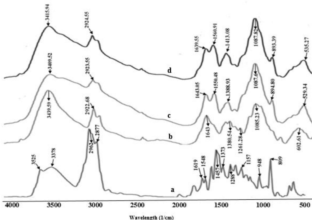
**Figure 1.** FTIR spectra of: (a) Thyme essential oil; (b) Chitosan powder; (c) Chitosan nanoparticle, and (d) Thyme oil loaded chitosan nanoparticle with chitosan: Thyme essential oil weight ratio of 1:0.4.
