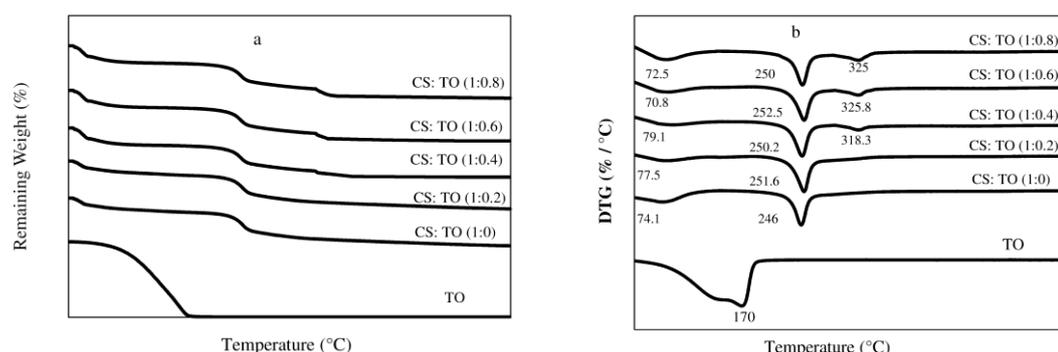
**Figure 2.** (a) TGA, and (b) DTG thermograms of Thyme essential Oil (TO), Chitosan Nanoparticle (CS-NP) and Thyme Oil loaded Chitosan Nanoparticle (CS-NP-TO) prepared using different initial weight ratios of Chitosan: Thyme essential Oil (CS:TO).
