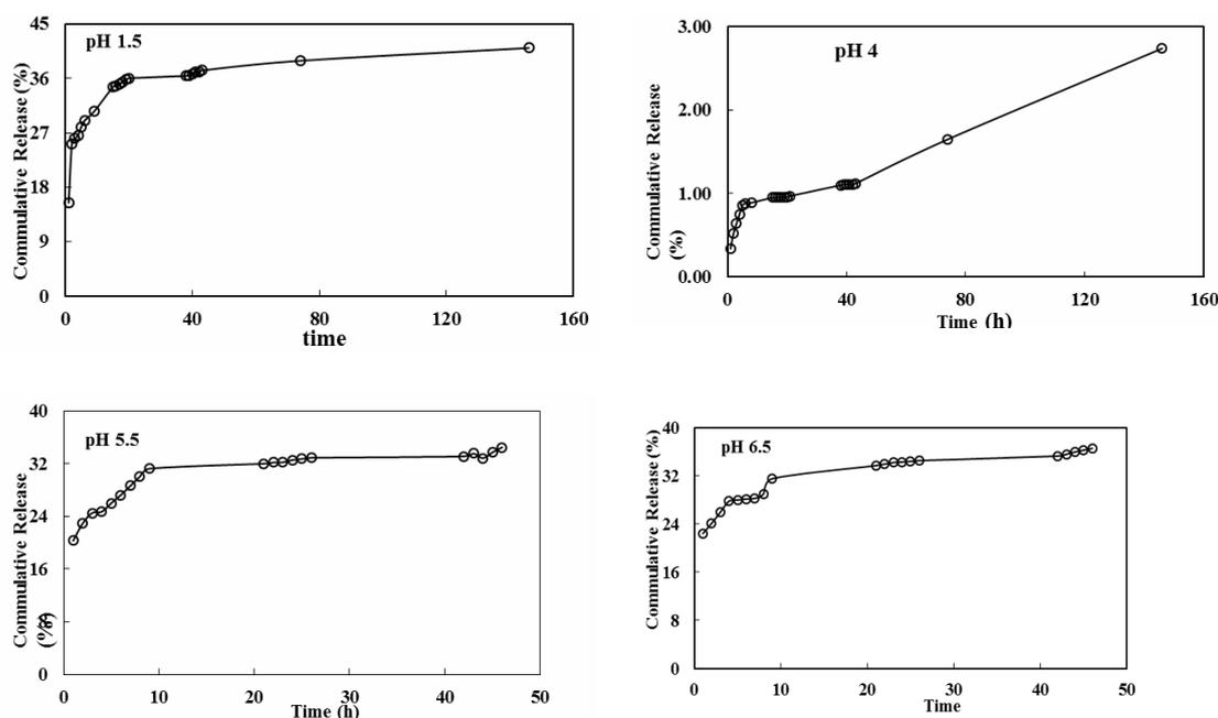
**Figure 6.** Release profile of GO from the GO/ $\beta$ -CD complex at different pH.
