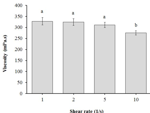
**Figure 1.** Viscosity as a function of shear rate of Poly Vinyl Alcohol (PVA)/Zataria Oil (ZO) dispersion. The apparent viscosity of the dispersion was measured using Brookfield viscometer at different spindle (No. 02) rotational speed of 1, 2, 5, and 10 s<sup>-1</sup>. Increase in shear rate leads a decrease in the viscosity, thus, PVA/ZO dispersion had a non-Newtonian shear-thinning liquid behavior.
