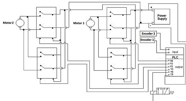
Figure 4. Electrical control circuit of the system.
