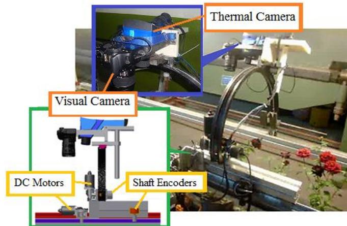
**Figure 1.** The developed automatic image capturing set-up.
