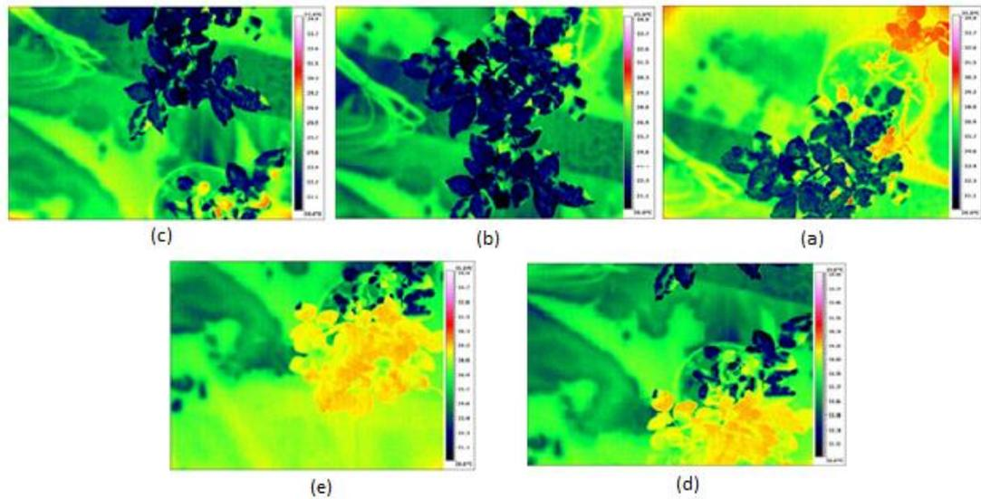
Figure 11. Thermal images of the specified positions at: (a) 90, (b) 100, (c) 110, (d) 120, and (e) 130 cm from the beginning of the longitudinal moving axis after the spray operation.
