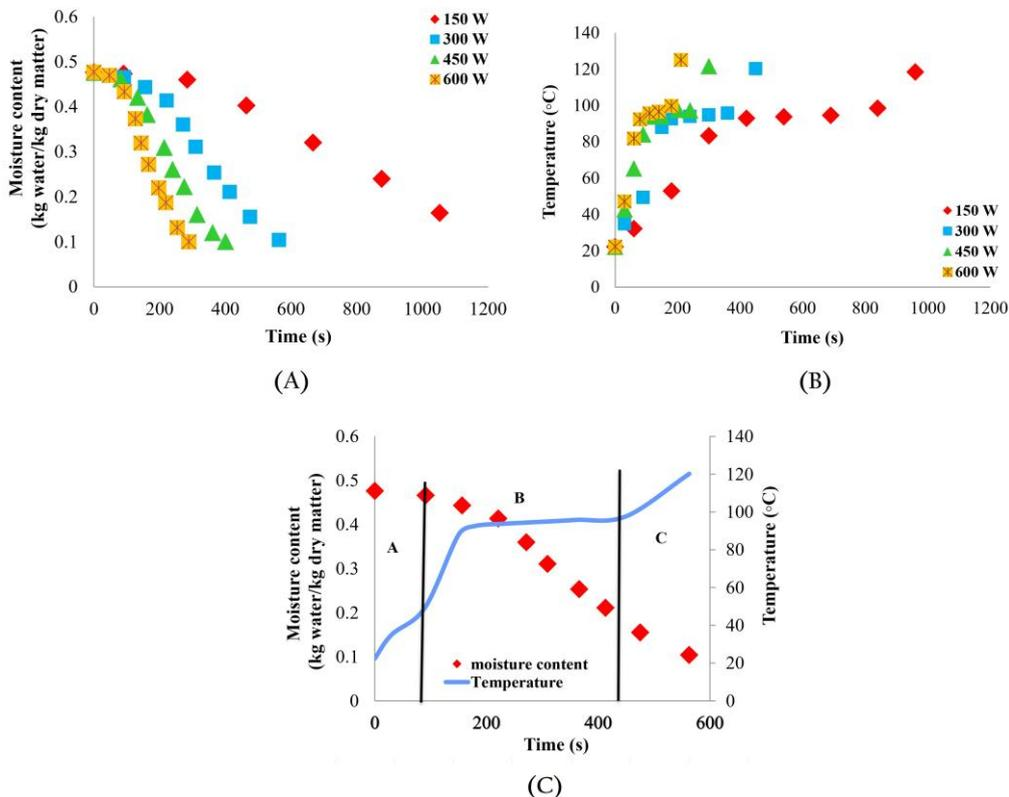
**Figure 1.** The moisture loss of samples during microwave baking (A), temperature profiles of cupcake microwave-baked at different time and MW power (B), and moisture and temperature profile simultaneously (C).
