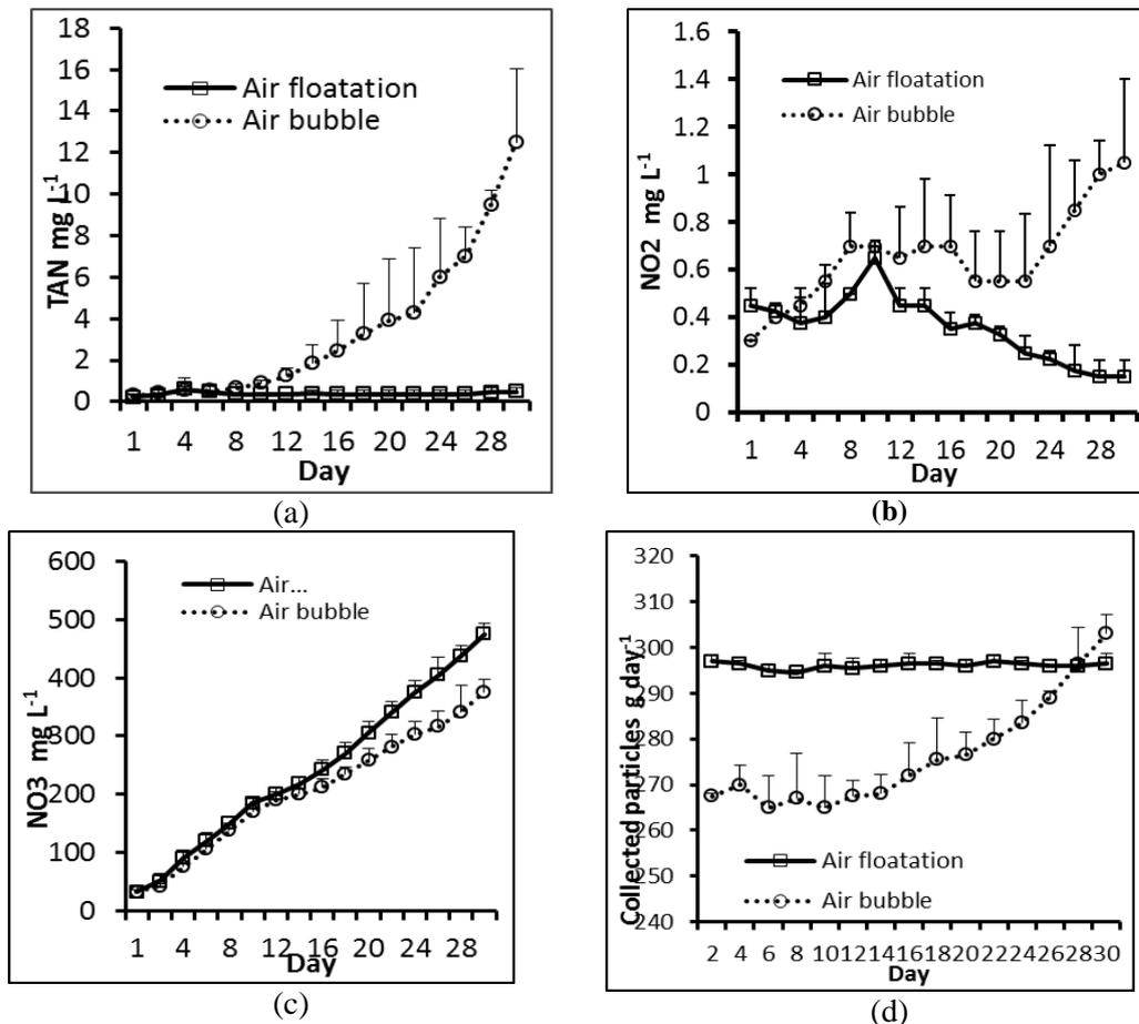
Figure 2. A comparison of Total Ammonium Nitrogen (TAN; a), Nitrite (NO<sub>2</sub>; b), Nitrate (NO<sub>3</sub>; c) and collected particles (d) in recirculation system as affected by two types of air bubble procedure (dissolved air floatation reactor versus a commercialized air bubble producer).
