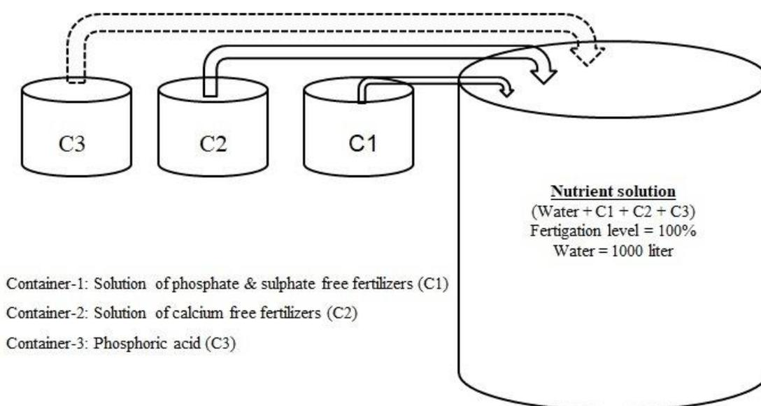
**Figure 3.** Preparation of nutrient solution for one level of fertigation (100%).
