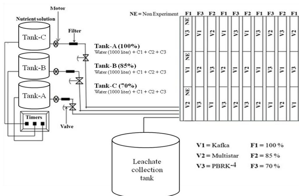
Figure 1. Schematic of experimental trial including fertigation system.
